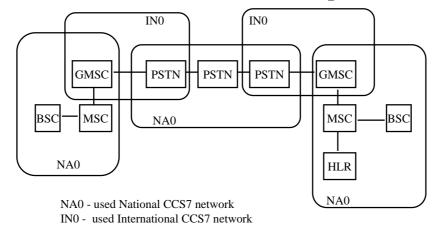
Signaling Point Codes are unique only in one signaling network!!
