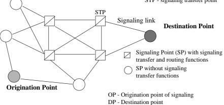
Examle: In Finnish CCS7 no specialized STP -nodes were originally deployed. STP functions were integrated in exchanges. In USA, China etc, specialized STP-nodes are commonplace.
