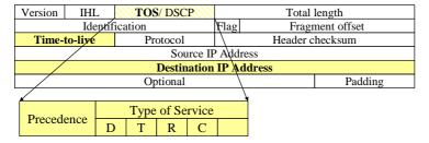
TOS = route selection criteria: D - minimization of delay or T - maximization of bandwidth or
