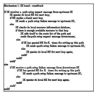
Fig. 4. Mechanism 1: SE based - crankback
