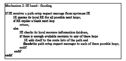
Fig. 5. Mechanism 2: SE based - flooding
