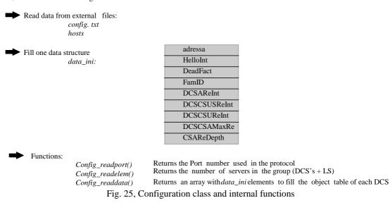
From these files we form the array with the addresses of all the servers which compose the SG. During the program implementation, we have tried to follow a modular way of working, and in Figure 26 we can see that in the configuration module this is also the case.
