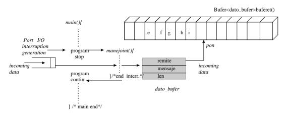
Fig. 17, Data management from the I/O port to the data buffer with the interruption handler
