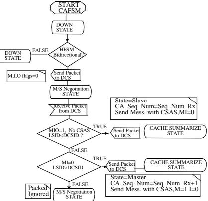
Fig. 5 Cache Alignment Finite State Machine (Master/Slave Negotiation)
