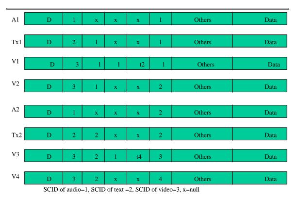
Figure 7: RMTP data packet formats.
