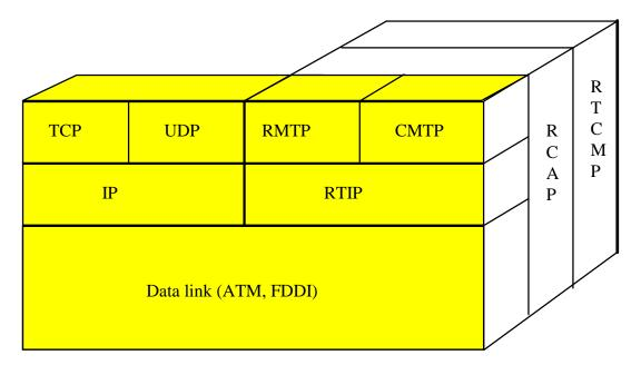
Figure 18: The Tenet real-time protocol suite.
