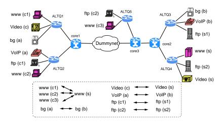
Figure 2.2: Measurement network topology.
