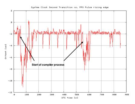
Figure 2.4: Clock offset from the PCI-based synchronization system in heavy I/O situation
