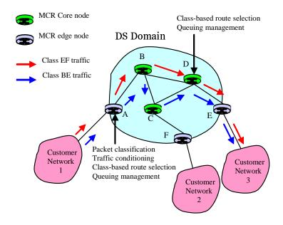
Figure 5.1: An example of the MCR DiffServ network
