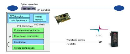
Figure 3.1: Measurement architecture
