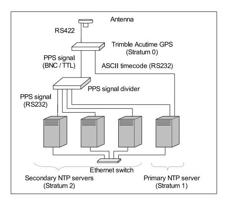
Figure 2.3: Architecture of GPS based time synchronization unit
